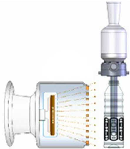
Bottle sterilization by electron beam irradiation ©Courtesy Frank-Holm Roegner
